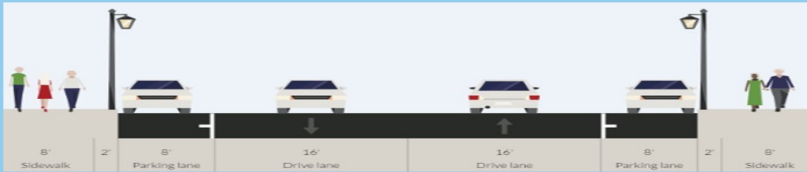
Existing – Typical Section
